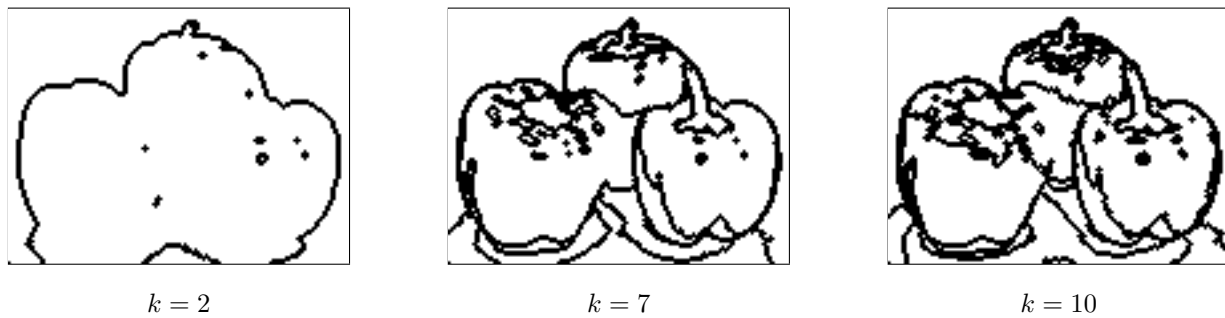
Fig. 8. Image segmentation results in the case of “paprika” image using k -means method ( k = 2, 7, 10 ). RGB is used as the color space. The black lines in the images indicate the boundaries of the regions.
