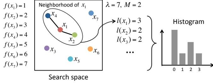
Fig. 1: Conceptual image of the procedure for calculating the LLP feature.  $\lambda$  and  $M$  indicate the size of candidate solution sample  $X$  and the neighborhood size, respectively.
