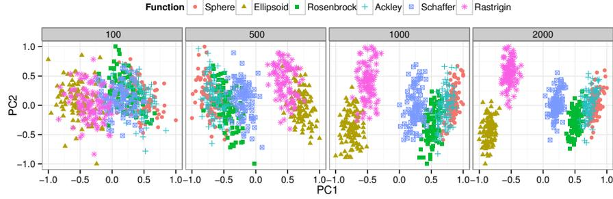
Fig. 3: Two dimensional plots using first and second principal components of the LLP feature vectors extracted from the 20 dimensional benchmark functions with the varying sample size  $\lambda = 100, 500, 1000, 2000$ . The 100 different sets of candidate solutions with the same size are generated for each function.
