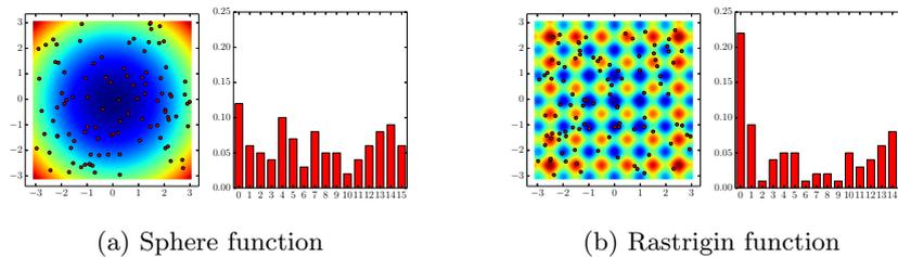
Fig. 2: Visualized fitness landscapes and the sampled candidate solutions for calculating the LLP feature (left), and the histogram of the LLP (right) on (a) Sphere and (b) Rastrigin functions, respectively.
